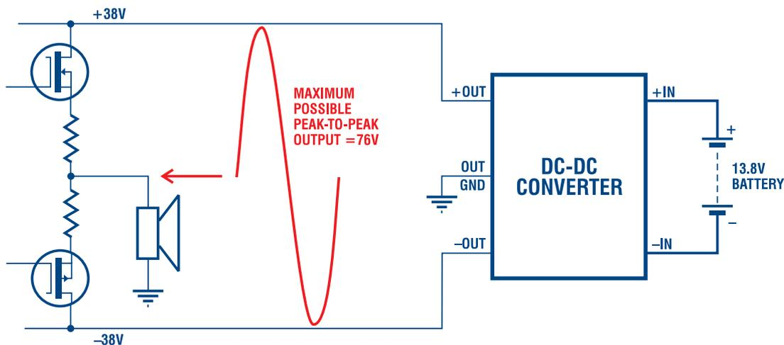
Fig.3: The only way to get REALLY high power output with a battery supply is to use a DC-DC converter to step up the battery voltage to a much higher value, so that the maximum peak-to-peak output voltage can be as high as we wish...
