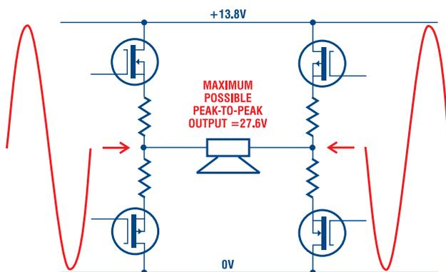
Fig.2: One way to get more output from an amplifier running from low voltage DC is to use a bridge-mode output stage. With each side of the speaker driven by opposite-polarity signals, the maximum peak-to-peak output now becomes TWICE the supply voltage.
