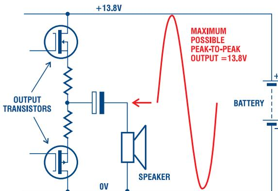
Fig.1: When an amplifier with a standard 'series push-pull' output stage runs from 13.8V DC, this becomes the absolute maximum peak-to-peak output.
