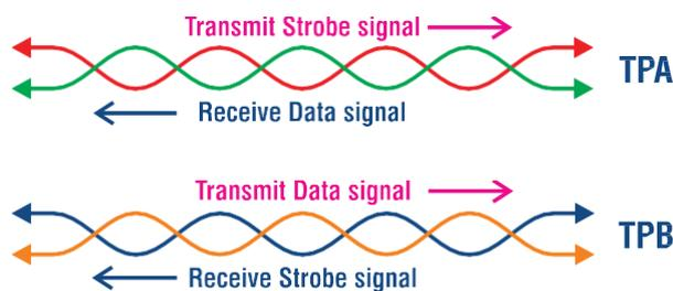
*Fig.3: The Strobe and Data signals are sent along the IEEE 1394 bus via two shielded twisted-wire pairs, TPA and TPB.*
