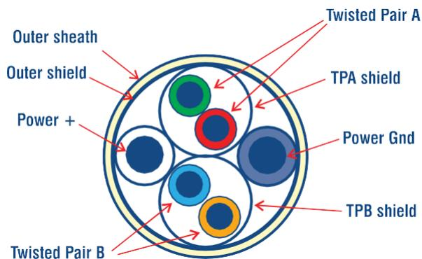
*Fig.4: The primary type of IEEE 1394 cable has a pair of power conductors as well as the two shielded signal pairs TPA and TPB.*
