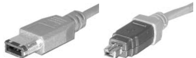
*Fig.6: The two different types of IEEE 1394 plug. The 6-pin plug is on the left and the 4-pin plug is on the right.*
