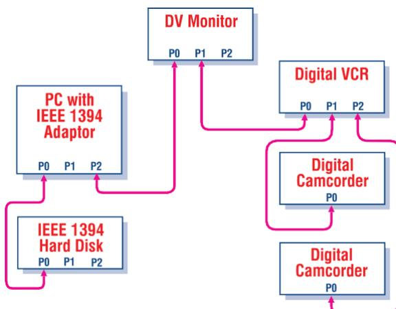
*Fig.1: A fairly typical IEEE 1394 network used in a digital video editing studio. The PC would generally take the role of bus manager and isochronous resource manager.*
