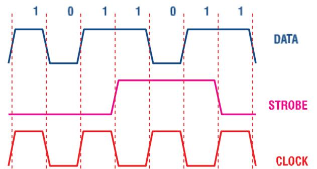
(Clock signal reconstructed at receiver by exclusive-ORing Data & Strobe signals)
