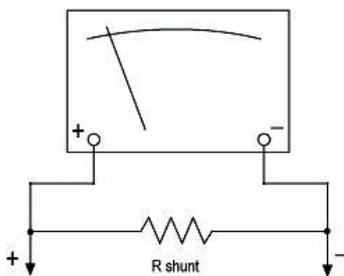
*Fig 1. Moving coil ammeter:
