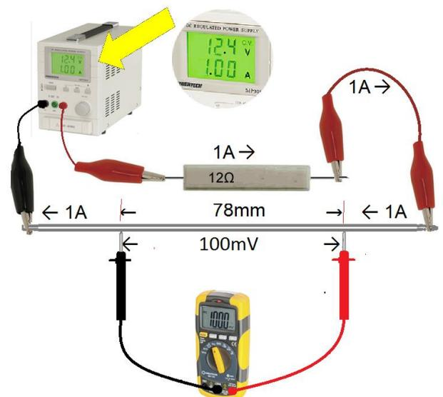
In this example, a 78mm section of resistance material (eg brazing rod, resistance wire, brass strap etc) was found to produce a 100mV voltage drop when 1 Amp is passed through it. (Here we show a power supply with an accurate built-in Ammeter, and the voltage is adjusted so that the Ammeter reads exactly 1 Amp. With the 12Ω shown, that would require about 12 Volts).
