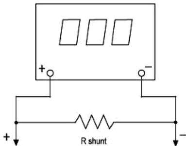
**Fig 3. Digital ammeter:**
