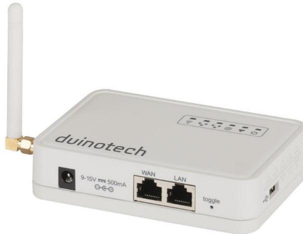
The XC4394 LoRa Gateway incorporates a OpenWRT based router SoC offering WiFi, LAN, WAN and USB connectivity. Also connected to the SoC is an ATmega328 microcontroller offering functionality similar to an Arduino Uno. Many of the ATmega328's IO pins are broken out to a screw terminal header. The ATmega328 is also connected internally to a LoRa compatible module.
