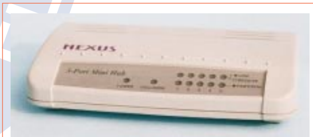
This very compact 10BaseT five-port hub is very suitable for small networks. One of its five ports can be configured as an 'uplink' port, with the connections internally crossed over. Power comes from a small 'plug pack'. The Nexus unit shown is sold by Jaycar stores as YN-8070.
